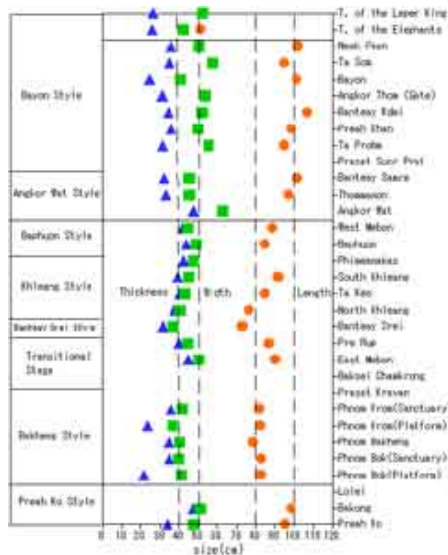
Fig. 2.6-5 The change in the size (thickness, width and length) of the sandstone blocks by age in the Angkor monuments (older to younger monuments from the bottom to the top).
